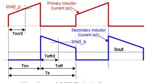
**Waveform of CCM Flyback Converter**
