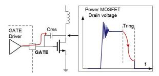
transformer demagnetization time corresponds to the inversion of the current by detecting this point, as shown in Fig. on the right.
