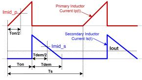
**Waveform of DCM Flyback Converter**
