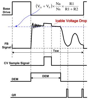
is a step at FB pin in the transformer demagnetization process, where Vo and VF is the output voltage and diode forward voltage; R1 and R2 is the resistor divider connected from the auxiliary winding to FB Pin, Ns and Na are secondary winding and auxiliary winding respectively.
