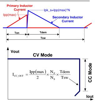
In CT5502S, the ratio between Tdem and Tsw in CC mode is 4/7. Therefore, the average output current can be expressed as:
